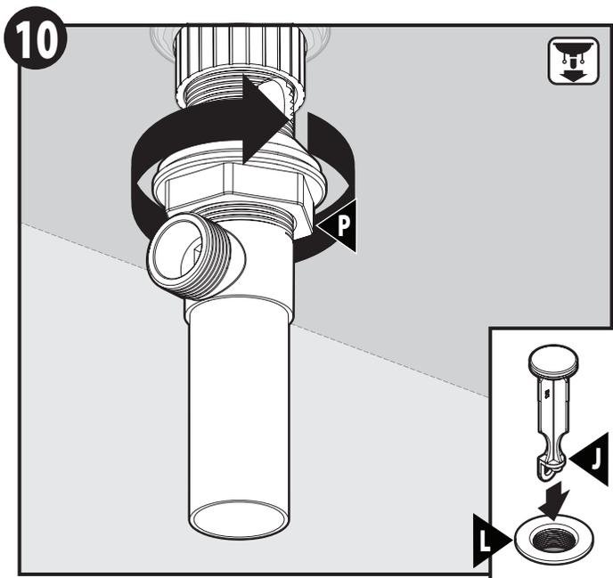
Tighten drain nut (**P**) and drop plug (**J**) into waste seat (**L**) as shown.
