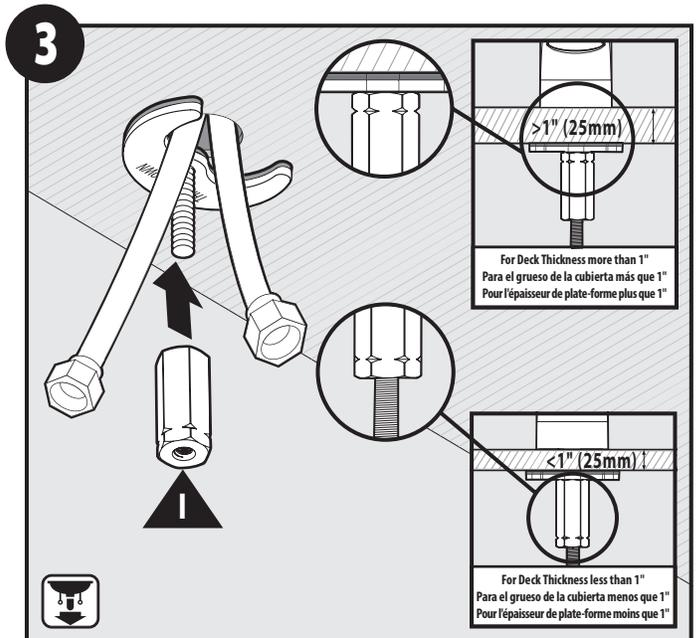
For sinks thinner than 1" attach the mounting nut (I) with the smaller end up as shown. For sinks thicker than 1" attach the mounting nut (I) with the larger end up as shown.
