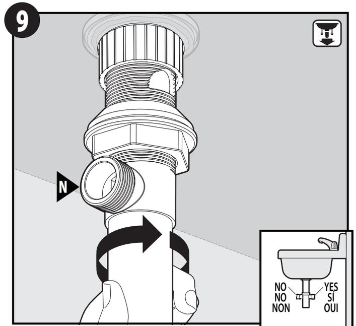
Rotate pivot rod opening on side of drain body (**N**) to face towards wall as illustrated.
