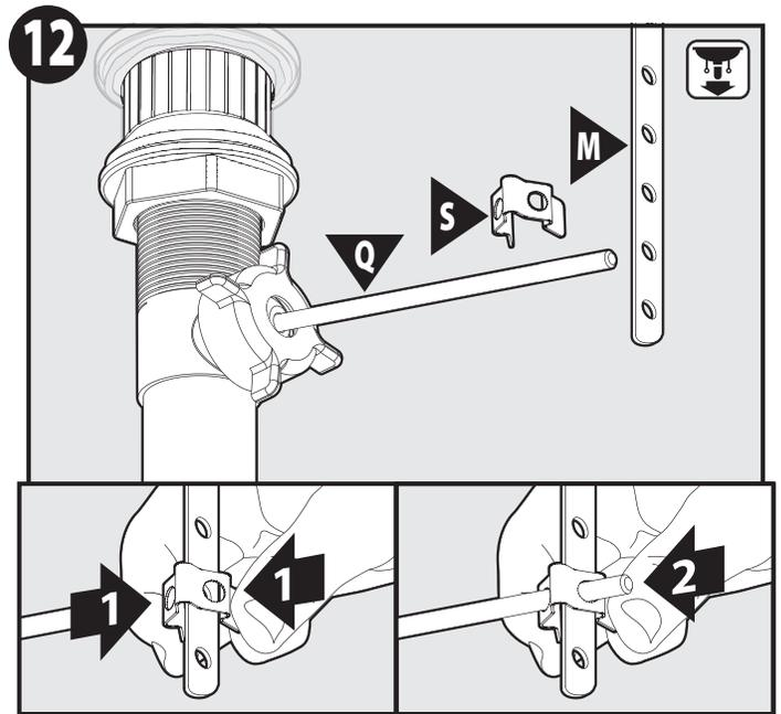
Push pivot rod (Q) down. Slide one side of clamp (S) onto pivot rod. Insert pivot rod through closest hole on strap (M) with pivot rod down. Squeeze clamp and slide other side of clamp onto the pivot rod.
