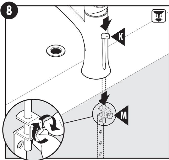
Install lift rod (**K**) into opening on the top of the faucet. Slide the lift rod strap (**M**) onto lift rod and tighten the bolt finger tight. Final tightening will be completed during Step 13.
