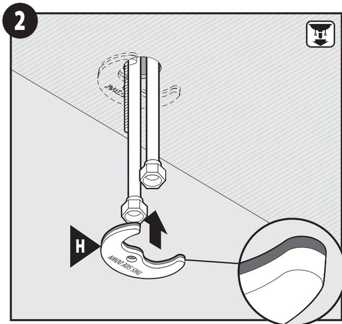
From below the sink, slide the mounting bracket (H) onto the threaded shank.
