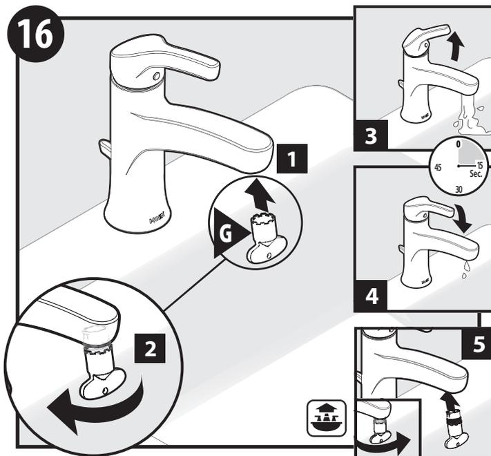
Flush debris from the plumbing system by removing the aerator by hand or by using the included aerator tool (G) provided with select models. Run hot and cold water for 15 seconds. Replace the aerator.
