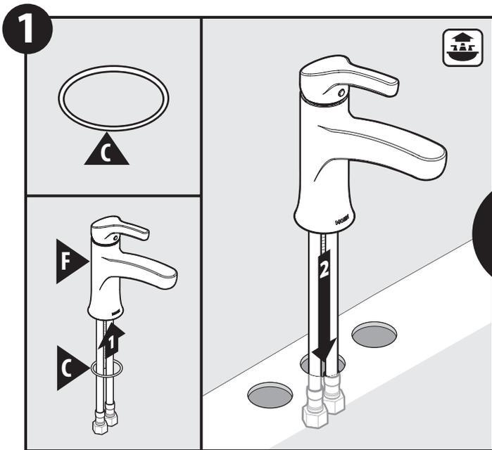
For single hole installations, place deck gasket (C) on the underside of the faucet body (F). Insert faucet into sink opening.
