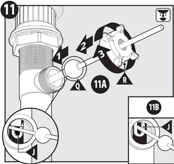
The pivot rod (Q) can be installed in two ways. Illustration (11A) shows the pivot rod (Q) next to hole in plug (J). This allows the plug (J) to be pulled out for cleaning. Illustration (11B) shows the pivot rod (Q) inserted into the hole in the plug (J). This prevents the plug (J) from being easily removed after installation. Once the pivot rod is installed (11A or 11B), tighten the pivot rod nut (R).
