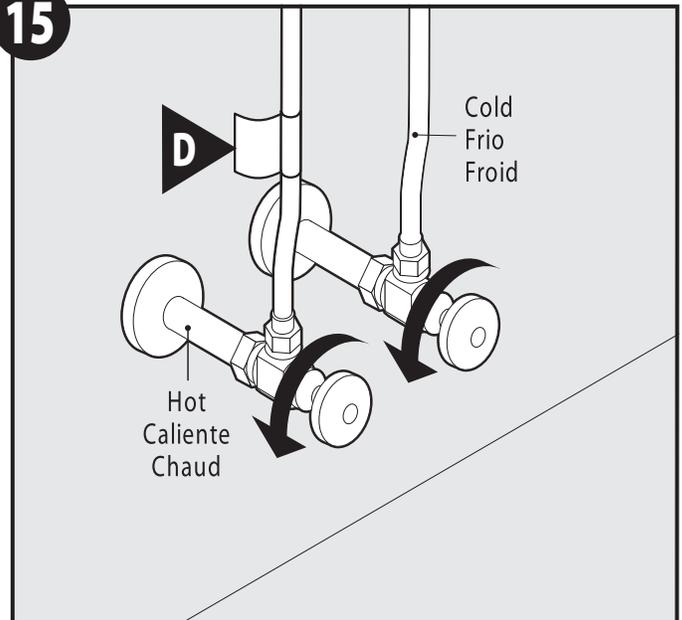
Turn on the water supply line valves on and check for leaks. Attach the Product Identification Label (D) in a conspicuous location such as on an inlet supply line.
