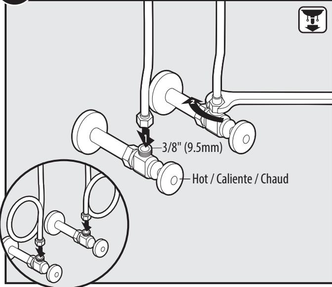
Attach the hot supply on the left side to the hot water shut off valve and tighten with a wrench. Do not use thread seal tape. Repeat these steps for the cold side. If the supply lines are too long, looping is acceptable.
