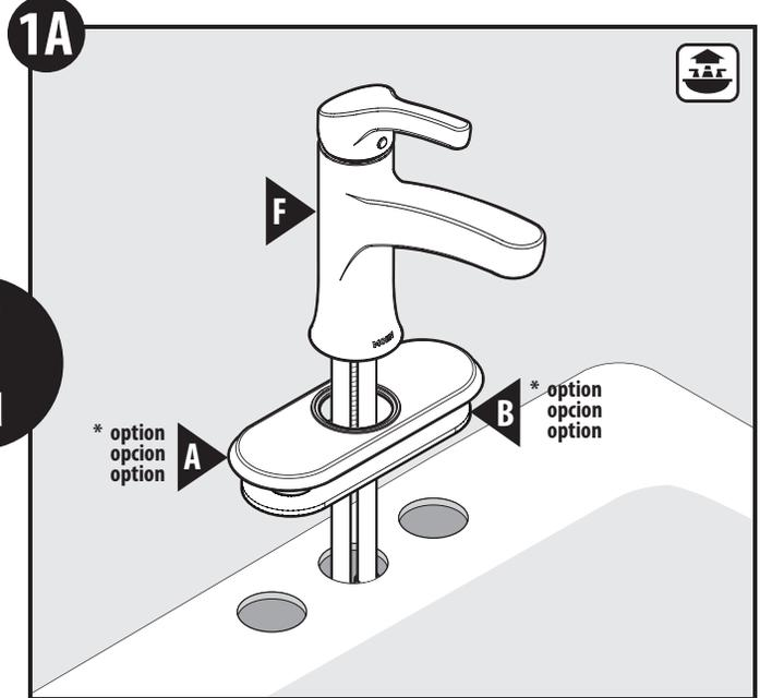
For 3 Hole Applications: Insert foam gasket (B) into underside of the deck plate (A) onto sink and insert faucet body (F) into opening.
