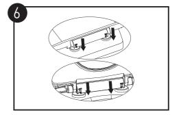
**重新安装盖板:** 沿支架柱方向将盖板支架孔扣入支架柱。 To reinstall the seat, buckle the seat bracket hole into the column along the direction of the column.
