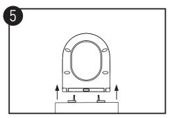
把盖板打开到垂直位置,然后用一只手垂直往上取出即可。 Open seat to vertical position, then lift the seat straight up with one hand.
