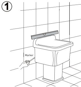
Move the mop sink and pedestal assembly to the installation place, make sure that the back of the mop sink fits the wall, and use a marker to mark the outline of the mop sink on the wall.
