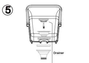
Install the drainer as shown in the figure; then hang the sink on the wall, check the level and the fit with the wall again, and check the fit between the pedestal and the sink. When there is no problem, finally fix it and apply anti-mold silicone on the gap between the wall and the ground.
