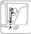
Pull out the filter from connector.
