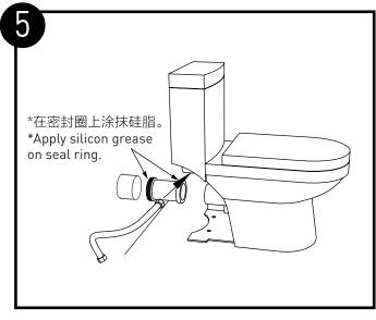
安装排污连接直管,并将供水软管一端与进水阀连接。 Connect the waste pipe, and connect supply hose to inlet valve of toilet.
